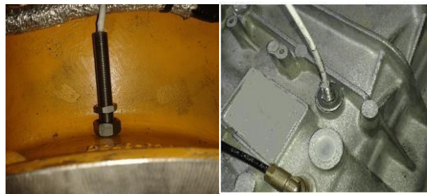
Figure 6. NVH test equipment fittings during truck torsional vibration testing [14]
