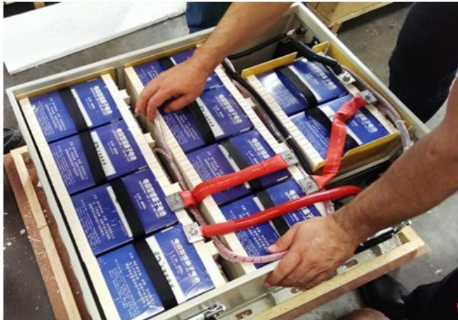
Figure 3: Example battery pack made with prismatic cells
