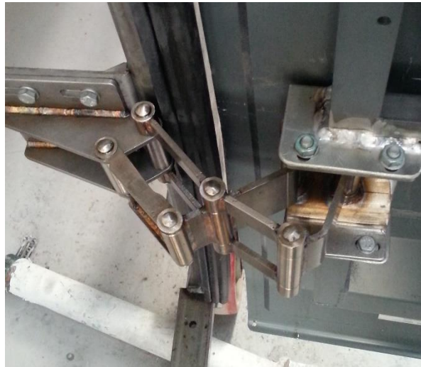
Fig. 11. New mechanism assembly on tailgate
